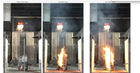
Figure 5-3: Photos of LFP fire development during intermediate-scale free burn test: near time of ignition (left), near time of predicted sprinkler operation (middle), peak heat release rate (right).
